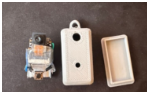
ESP32-S3 Sense module with camera (left), 3D-printed enclosure front (center) and back (right).
